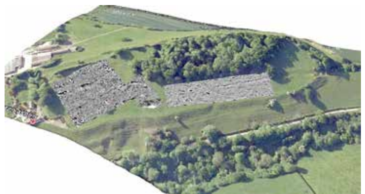
Digital Elevation Model of Google Earth satellite photograph, showing the survey results in topographic context [Geophysical Survey data overlain on Google Earth image, floated on ASCII LiDAR DSM (from Geomatics Group). Viewed from NNW, 1.4x vertical exaggeration].
